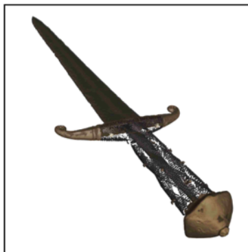
Fig. 2: The sword from lake Zug as seen with X-rays.
