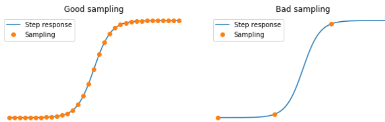
Fig. 4.4: Selecting the correct frame rate is essential to allow the study of a process.
