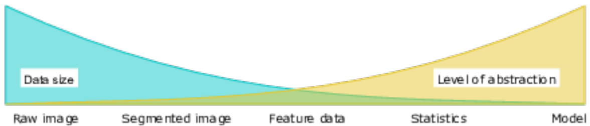
Fig. 9.2: The data size decreases radical when we increase the level of abstraction.
