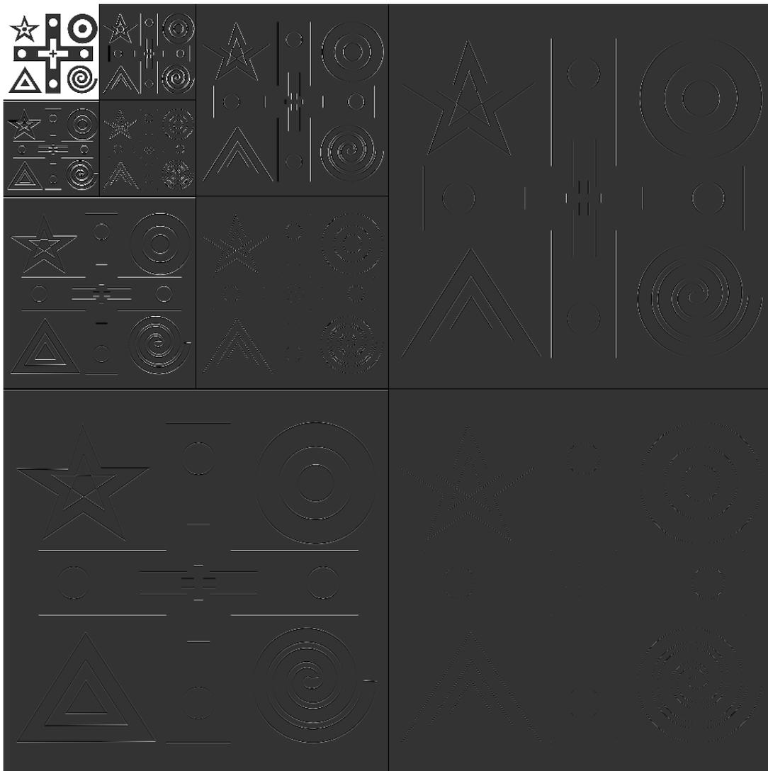
Fig. 7.5: Transform workflow for a 2D wavelet decomposition.
