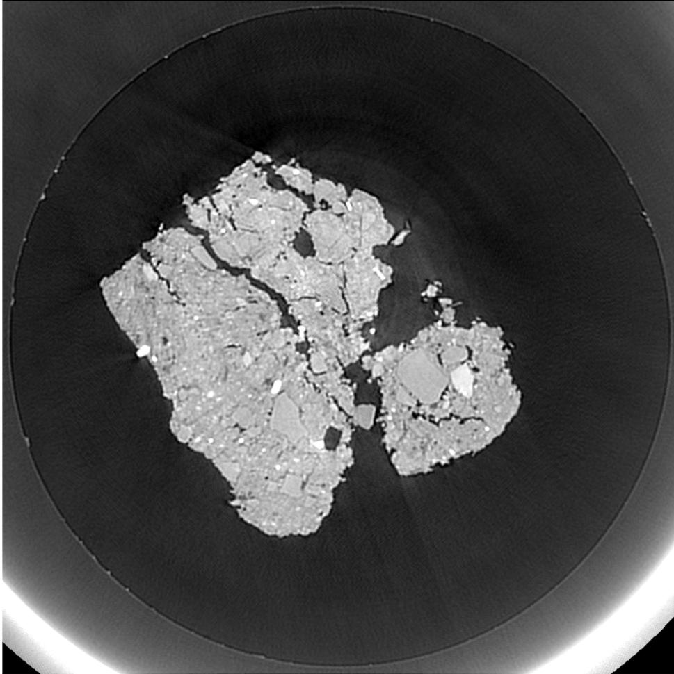
Fig. 6.2: CT slice after applying stripe removal filter.
