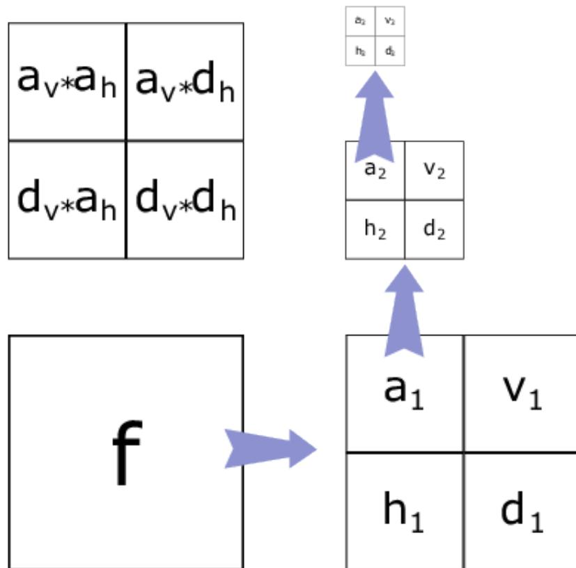
Fig. 7.3: Transform workflow for a 2D wavelet decomposition.
