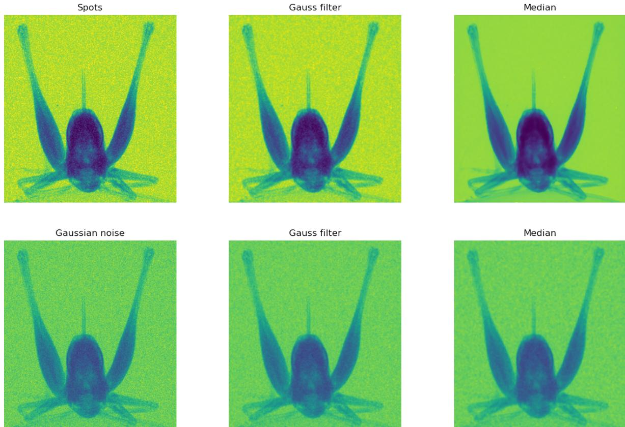
In this comparison, you can clearly see that the median filter is superior when it comes to remove outliers in an image. In this case, the Gauss filter is only smearing out the outliers, but they still appear as noisy.
