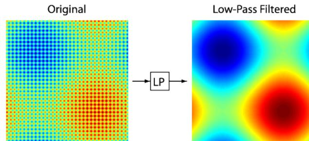
Fig. 4.1: The principle of a low-pass filter.
