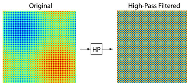
Fig. 4.2: The principle of a high-pass filter.
