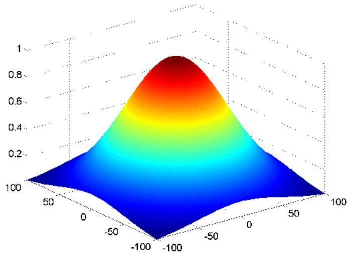
Fig. 5.1: The shape of a Gaussian filter kernel.
